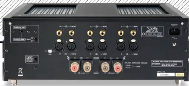
ABOVE: Three balanced (XLR) and three single-ended (RCA) line-level inputs may be reconfigured to operate the A-2 v2 in bridged/BTL mono mode and in 'power amp direct' mode. The single sets of 4mm speaker terminals serve all modes
