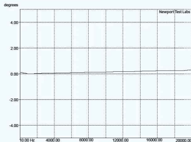
Graph 11. Interchannel phase response (24-bit/48kHz)
