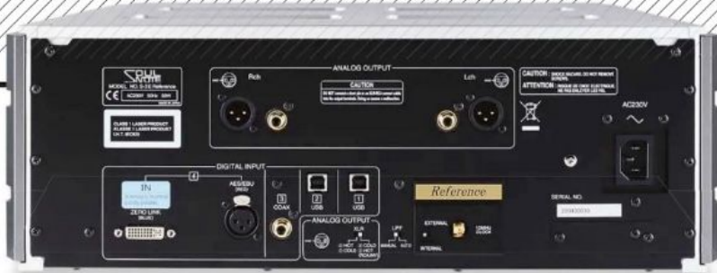
ABOVE: Digital inputs are on coaxial, USB-B (x2), AES/EBU and a proprietary 'Zero Link' port for use with compatible network transports. An external 10MHz clock is also supported. Outputs are on on RCAs and configurable, balanced XLRs
